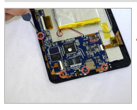
Using #00 Phillips Screwdriver, remove the four 1mm screws holding the circuit board to the device.
