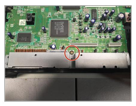
Remove the #1 Phillips Screw from back port cover, and then remove the cover.
