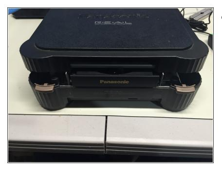
Remove the top portion of the case to expose the internal components.
