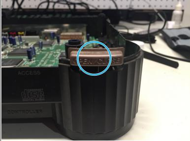
• Remove the plastic cover, power and eject buttons found at the front end of the unit.
