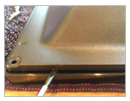
Once the screws are all removed, slide the flat-head screwdriver into the small gap between the front and back plates. Use the screwdriver to pry the plates apart and lift the back plate up.
