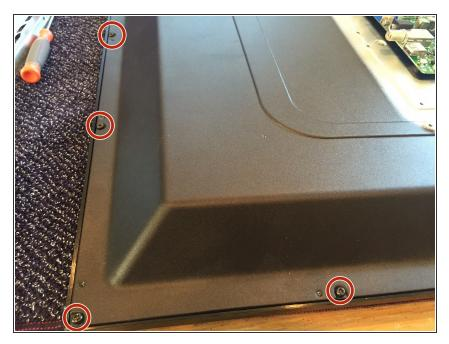
Remove all of the 18 screws connecting the front frame to the back of the TV with the Torx screwdriver.
